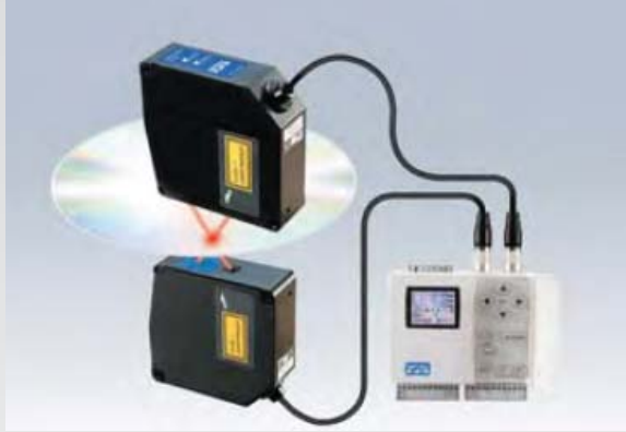
Two CD4-30 sensors are connected to 1 CD4A-N controller. The sensors are set-up to measure the thickness of the metal disk. The disk is positioned on a spindle and rotated. The Analog thickness data is taken out of the controller and stored in a PC.
