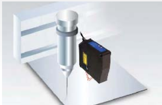
A small amount of glue is evenly coated on a metal surface. The CD4 series is set to measure the thickness of the glue to verify even distribution on the metal part.
