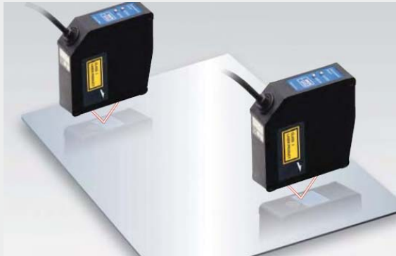
The CD4-L25 transparent measurement version is looking at a very shiny mirrored glass surface. The CD4-L25 measures 2 locations on the plate and if the distance is out of tolerance the plate fails inspection.
