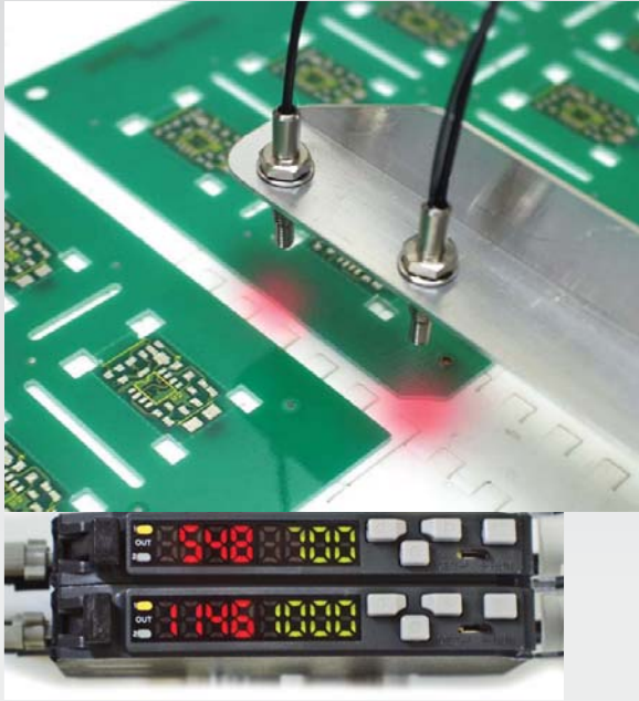
Two D2RF sensors and 2 diffuse M4 fiber cables verifying the correct orientation of a circuit board on a conveyor line. By positioning one fiber cable at the location of the notch and one placed slightly higher to detect the leading edge of the board, the amplifier can easily determine proper orientation of the boards.
