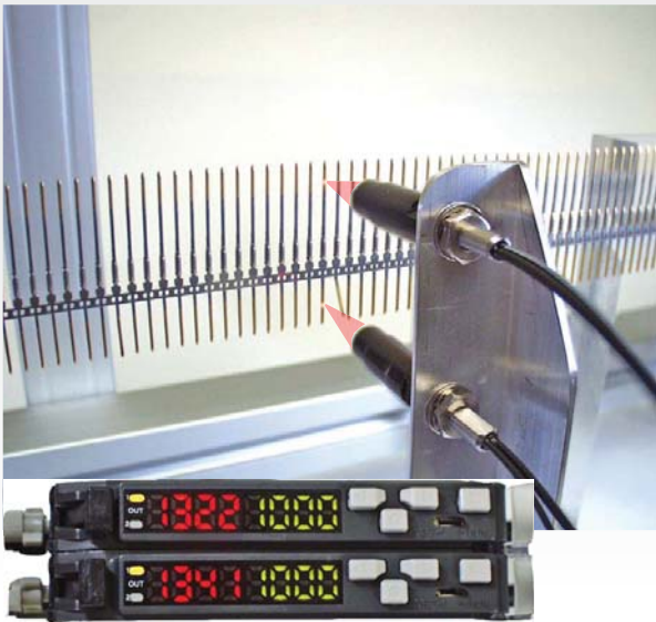
Two D2RF sensors and 2 diffuse fiber cables with focusing lenses checking for missing or bent pins. The pin point beam is less than 1 mm in diameter making it easy to detect the small pins.
